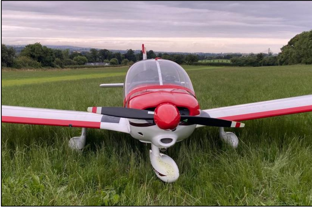
Photo No. 2: Photo showing distortion to nose landing gear ( courtesy of the Pilot )
